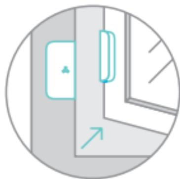
The sensor sends signal to Aqila Securehub™ when the magnets attached to the sensor move away from the main part. Tamper protection ensures that any attempts to remove the sensor which will activate the alarm.
